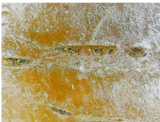
Figure 4. Photo of the surface of etrol sample No. 1 after 140 days of exposure in active soil at 60X magnification.
