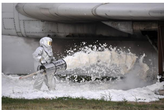
Figure 4. Fire extinguishing method using fast-solidifying non-combustible mineral foam.
