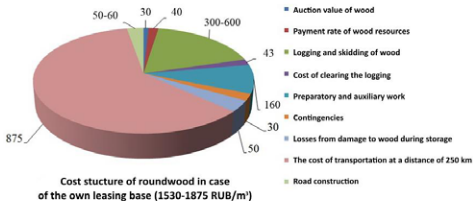
Fig. 2. Cost structure of roundwood in case of the own leasing base, RUB per m 3 (Tambi et al. 2017).
