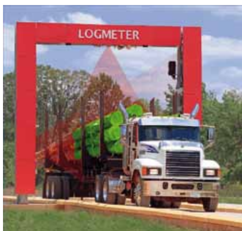
Fig. 6. An automated scanning system (Logmeter) to estimate biometric characteristics of logs (WoodTech 2021).
