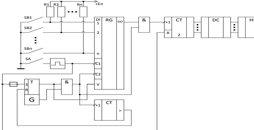
Fig. 10: Functional Diagram of Digital Device Intended for Counting Open/Closed Contacts
