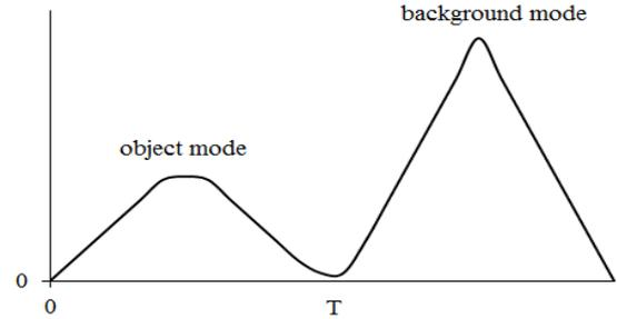
Fig. 2: A Threshold Value on a Bimodal Histogram
