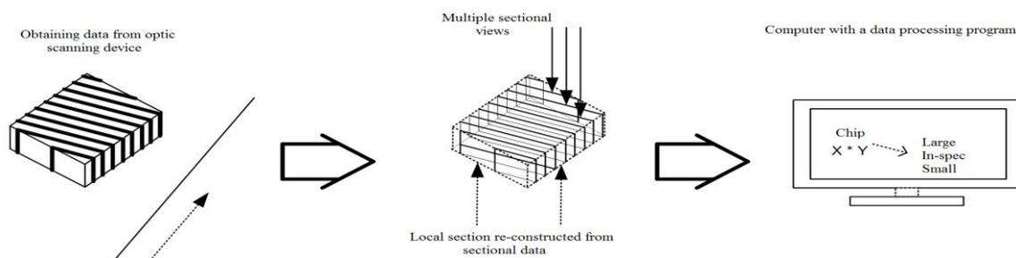
Fig. 7: Process Sequence of Given Feedback System
